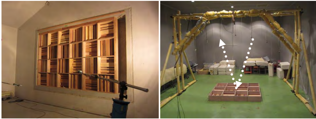
Figure 3. Measurement setups for absorption and oblique incidence absorption coefficient
