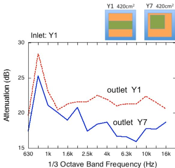
**Figure 4** Measured results of SPVG with outlets Y1 and Y7. Good agreement with our theoretical prediction.
