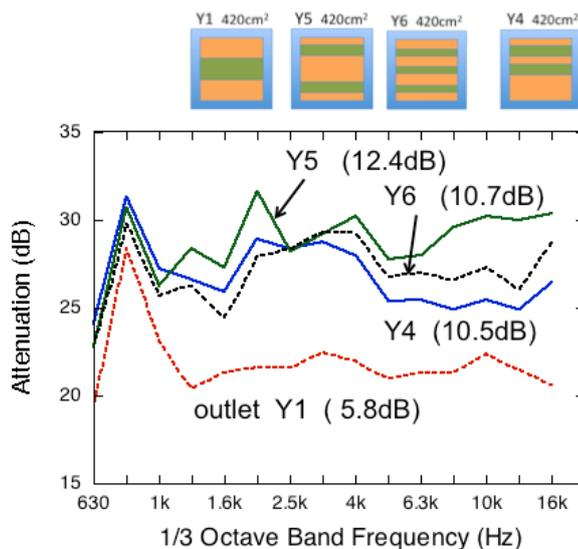
**Figure 5** Measured results of SPVG with change of outlet's number
