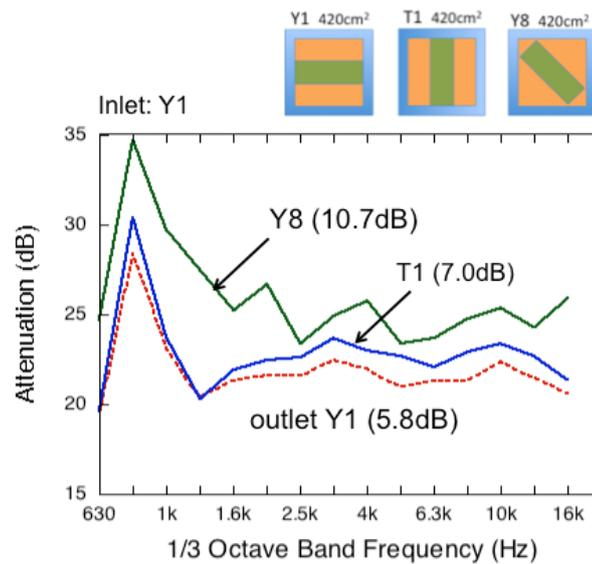
**Figure 6** Measured results of SPVG with change of outlet's direction
