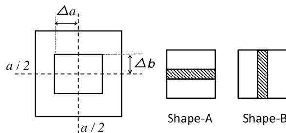
**Figure 2** Coordinate system to find a reasonable shape of inlet and outlet
