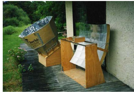
Figure 2 Solar oven in the left and solar cooker in the right
