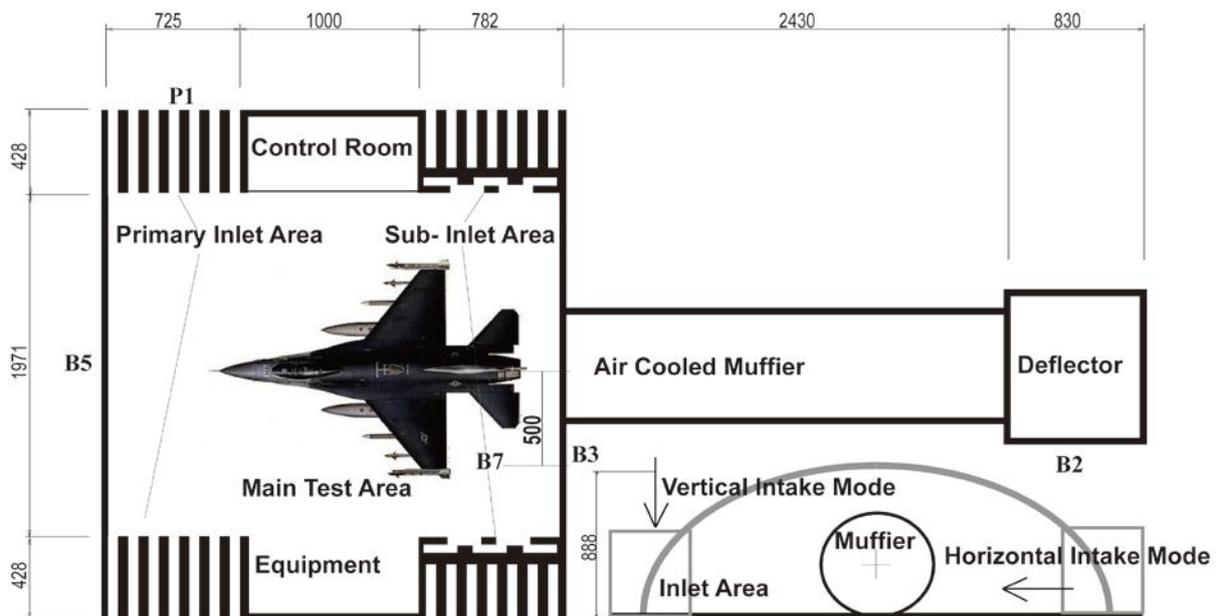
**Figure1.** Locations of noise survey stations and the current T-10 hush house arrangement at near-field
