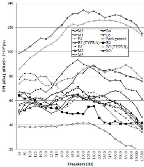
**Figure5.** The spectrum of each diagnosed location, in afterburner mode.
