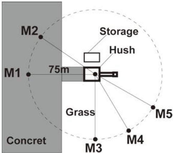
**Figure2.** Locations of noise survey stations (M1 ~ M5) and the current T-10 hush house at far-field
