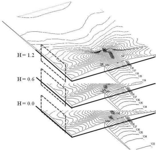
**Figure4.** The boundary noise levels at the inner side of the inlet area simulate a side wall at every 0.6 m height.
