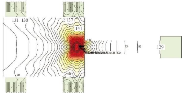
**Figure7.** The noise distribution at the near field is simulated using the remodeled T-10 for aircraft TYPE-A, in afterburner mode.
