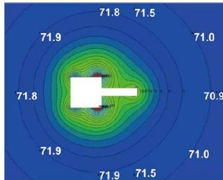
**Figure8.** The noise distribution at the far-field is simulated using the remodeled T-10 for aircraft TYPE-A, in afterburner mode.
