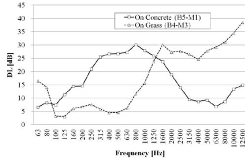
**Figure6.** The differences between on concrete and grass of each diagnosed location, in afterburner mode.
