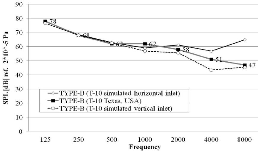
**Figure9.** Comparison between the measured and calculated SPL values for aircraft TYPE-B installed in the current T-10.
