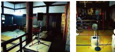
Fig. 6 L) Sound source and R) microphone at the measurement. The height of the speaker and dummy head is 0.9m.
