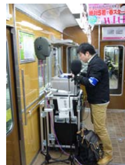
Fig. 1. Experimental apparatus – Dummy head microphone setup.
