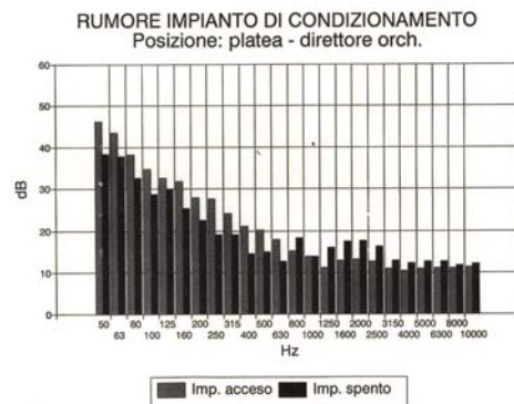
Fig.6. Frequency analysis of noise induced in the same position as Figure 5 from the Air Conditioning Plant located in the orchestra pit
