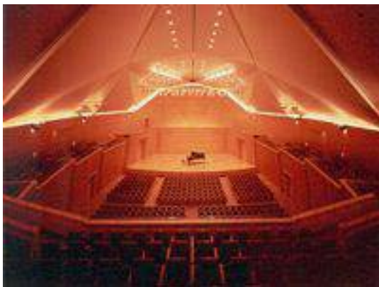
Photo 1. The Kirishima International Concert Hall, Kagoshima with tilt sidewalls and triangular ceilings.
