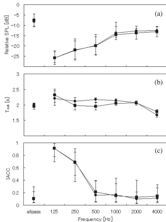
Fig. 2. The values of (a) relative SPL, (b)  $T_{sub}$ , and (c) IACC in 1/1 octave bands averaged for all measurement points in two halls (●: Tsuyama and ■: Kirishima).
