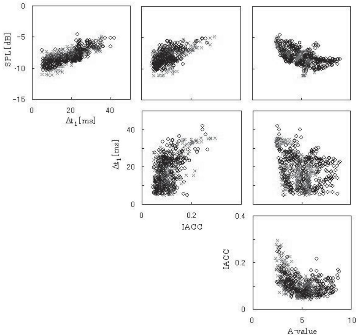
Fig. 10. Scatter plots between acoustical parameters SPL,  $\Delta t_1$ , IACC, and A-value for all values in O : Tsuyama and X : Kirishima
