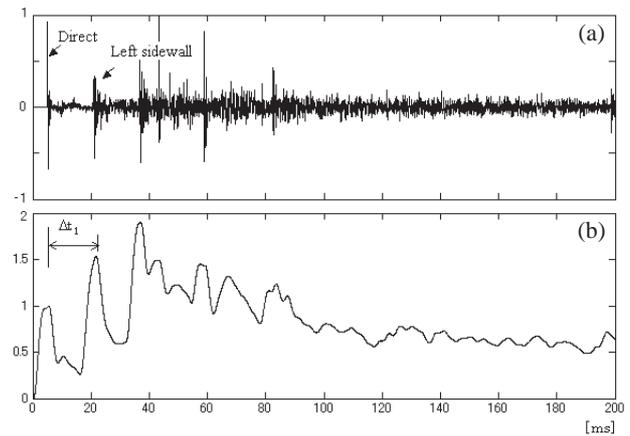
Fig. 6. (a) Example of the impulse response and (b) the integrated impulse response with integration time of 5 ms.
