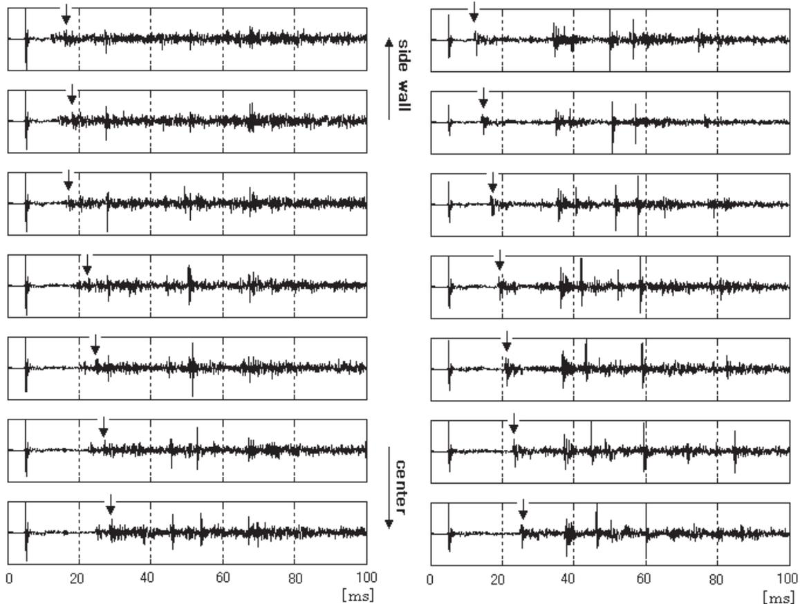
Fig. 8. Examples of left ear impulse responses measured at fifth rows of the audience seats in Tsuyama (left) and Kirishima (right). Arrows indicate the values of  $\Delta t_i$ .
